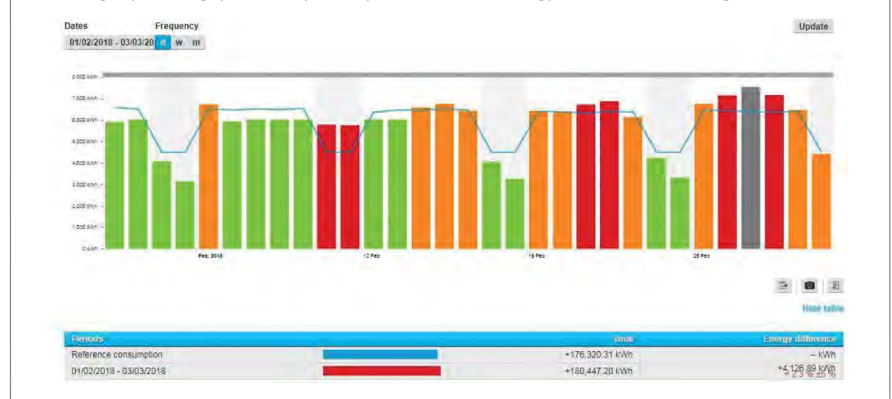
The 'traffic light' system is a highly effective daily check on performance in manufacturing plants and commercial buildings
