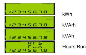
The Hours Run register accumulates the total time during which the average 3 phase load current exceeds a preset level. This is always displayed with a resolution 0.1 hour.
