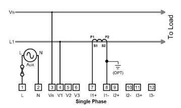
**CAUTION**: The instrument is internally fused at 250V 100mA. External fusing is required if the supply voltage exceeds 250V.
