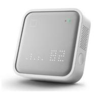
The "No Display" mode allows you to disable any information presented on Omni. Display modes are selectable via the device Settings in the Awair app. You can also swipe on the right edge of Omni's display to change the display mode, or press the Power Button to automatically cycle through Omni's real-time sensor readings.
