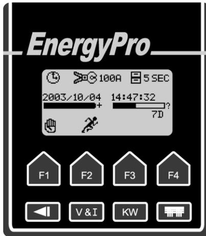
The **EnergyPro** will start recording on an even minute or half minute. While waiting for the recording to synchronize to the time the 'running' icon will be animated to 'run' on the spot. After the first record is recorded the 'running' icon will be animated to move across the bottom of the screen and the red 'logging' LED will flash.
