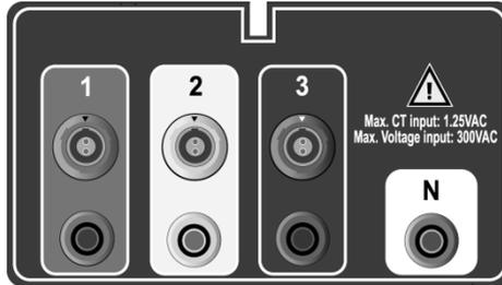
The voltage and current connections are colour coded according to individual phases.
