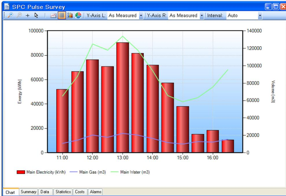
The above window shows the default view for the sample survey. Note that it is a dual axis graph showing energy in kWh on the LH axis and Volume on the right, and three data traces are present for electricity, water and gas (1 X bar chart and 2 X line chart traces). The bar chart is always referenced to the LH Y axis, and the line charts to the RH one.
