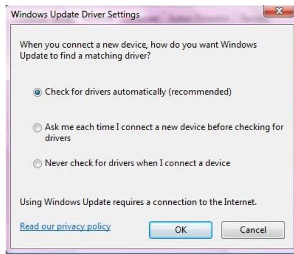
Ensure that 'Check for drivers automatically' is selected and reconnect your SPC device to a spare USB port. If the PC is connected to the web, the drivers will now load.
