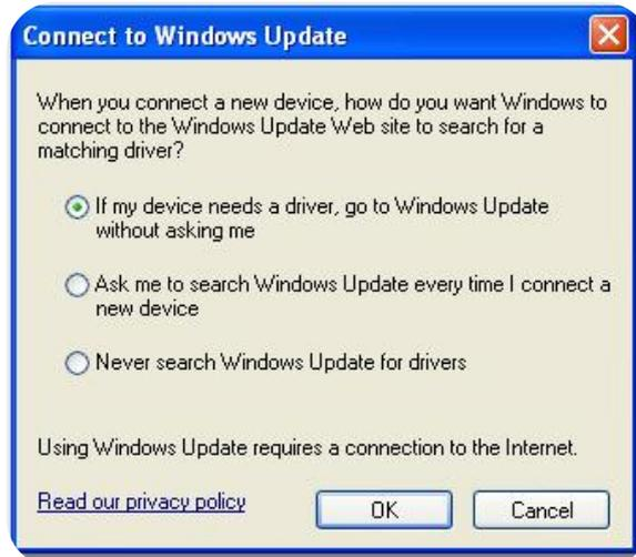
Select either of the first two options to enable Windows Update reconnect your SPC device to a spare USB port. If the PC is connected to the web, the drivers will now load.
