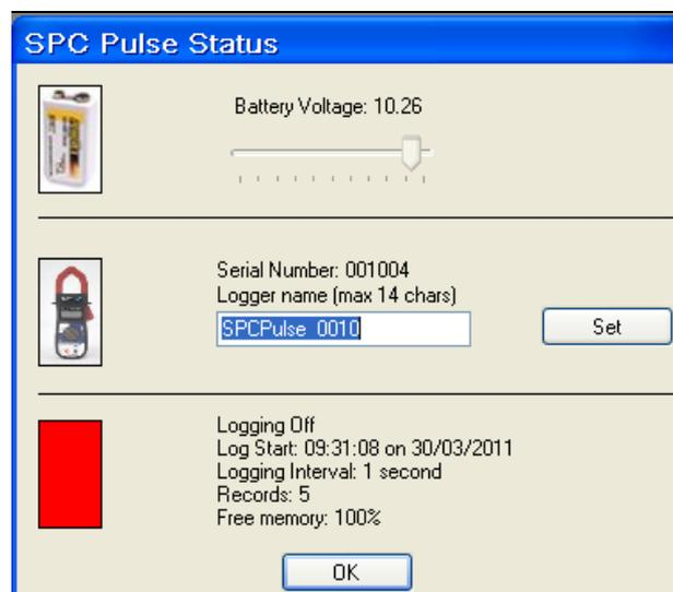
Details of the device and any recorded data are shown, along with the logging status indicator. Green for 'on' and red for 'off'. Note that the logger name can be set as desired.
