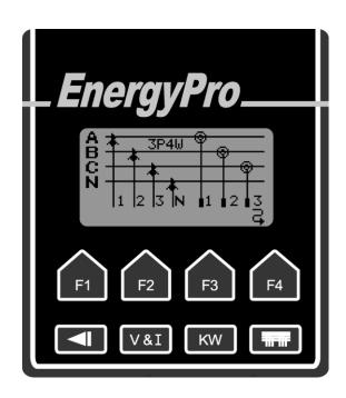
The hook-up screen will appear when the button is pressed. Before a survey is started this screen can be used to set the type of connection. There are five different connection types available: 1P2W, 1P3W, 3P3W, 2.5E and 3P4W. Press 'F4' to scroll through different connection types.
