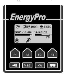
The *EnergyPro* starts recording on an even minute. While waiting for the recording to synchronize to the time the 'running' icon will be animated to 'run' on the spot. After the first record is recorded the 'running' icon will be animated to move across the bottom of the screen and the red 'logging' LED will flash.
