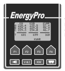
The Power screen will appear when the button s pressed. It displays real, apparent and reactive power for each phase.
