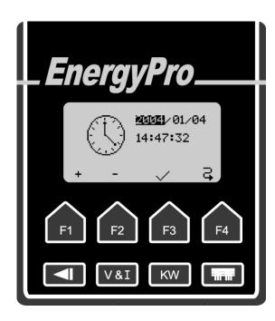
The clock setup screen will appear when the clock icon on the main screen has been selected. The scroll key (F4) is used to scroll through the fields: year, month, day, hour, minute or second. The + and - signs (F1 and F2) are used to increase or decrease the value. Press the checkmark key (F3) to confirm changes and return to the main screen.
