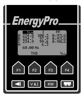
The voltage/current/power factor screen will appear after pressing the button. It displays RMS voltage, RMS current, and power factor for each phase. Switch between Line-to-Neutral voltage ( $V_{LN}$ ) and Line-to-Line voltage ( $V_{LL}$ ) by pressing F4. Note that  $V_{LL}$  is not present in the 1P2W configuration.
