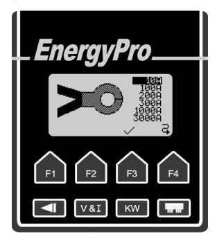
The CT setup screen will appear when the CT icon on the main screen has been selected. The scroll function key (F4) is used to select the desired CT range. The checkmark key (F3) is used to confirm the selection and return to the main screen.
