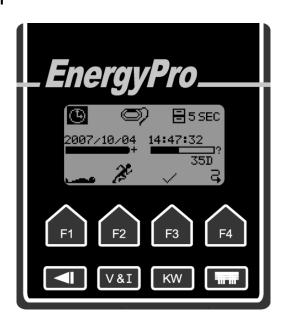
The main screen of the *EnergyPro* is a collection of icons that provide access to various configuration setup screens. It also displays general status of the logger such as battery charge state, available memory, and logging status.
