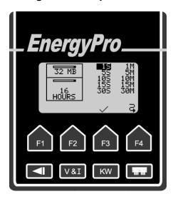
The storage rate setup screen will appear when the filing cabinet icon on the main screen has been selected. The scroll key (F4) is used to select the storage rate for the survey. The maximum survey duration, displayed in the lower drawer of the filing cabinet, will change when the storage rate is changed. The checkmark key (F3) is used to confirm the change and return to the main screen.
