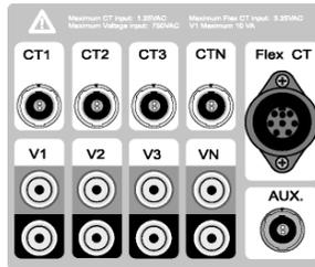
When measuring less than 3 voltages V1 must always be used. V1 zero crossing is used to synchronize the data sampling and measure frequency. In the event of an outage on V1 the logger has an internal digital phase lock loop that simulates the zero crossing until V1 is restored.
