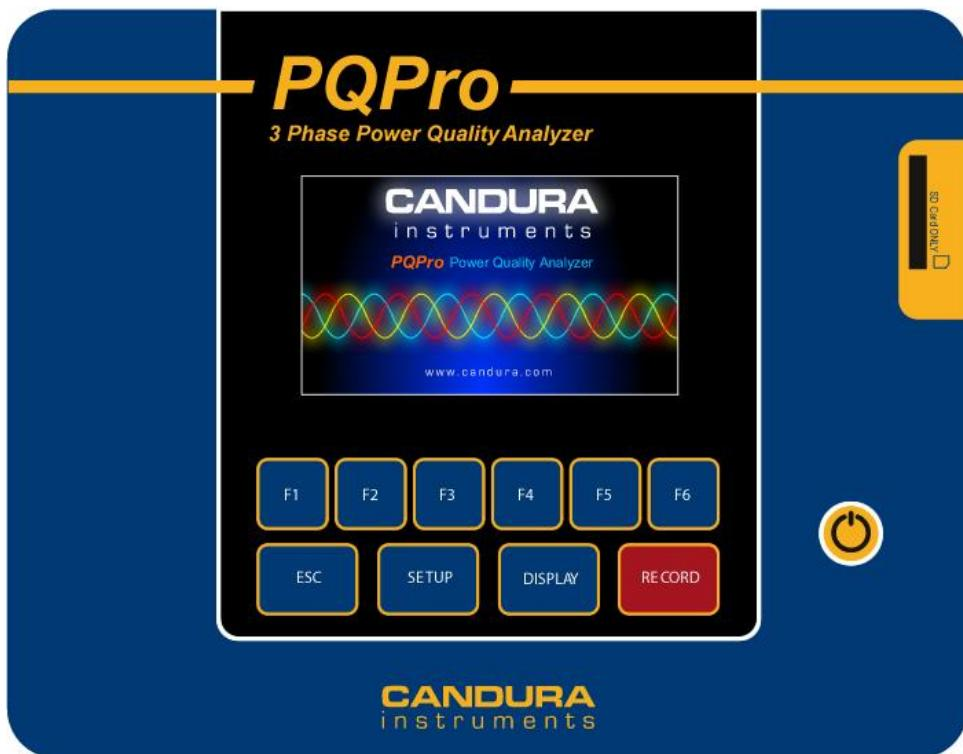
The memory card interface is used to store recorded data on a memory card and also to load new firmware. The **PQPro™** will not begin a survey without a memory card installed. Once a survey has been started the memory card may not be removed until the survey has been stopped.
