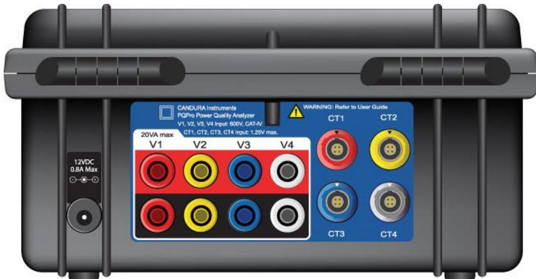
When measuring less than 4 voltages V1 must always be used. V1 zero crossing is used to synchronize the data sampling and measure frequency. In the event of an outage on V1 the logger has an internal digital phase lock loop that simulates the zero crossing until V1 is restored.
