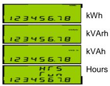
Press and together and hold for 2 seconds to reset the hours run register.
